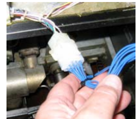
Figure 2: Connect the K3000 using the supplied harness.
